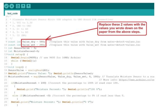
Save the code and upload it to the Arduino UNO.
