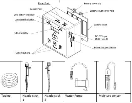
**Note:** You can't make any change in settings while the water pump is running, because the previous moisture in the setting was lower than the real-time moisture that the moisture sensor is detecting, if so, place the moisture sensor into the water while doing this setting, the water pump will stop running when moisture is 100%.
